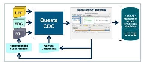
Using only your RTL (and SDC constraints or UPF power intent files), Questa CDC solutions automatically generate and analyze assertions to guard against chip-killing CDC issues. Metastability models can be exported to Questa Simulation for further analysis, and all results can be transmitted to the master verification progress database via UCDB.
